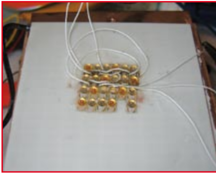
The first half of the LEDs has been connected together using thin klynar wire. Never use superglue to hold the wiring in place. Any repairs to loose wiring will then be made extremely difficult.
