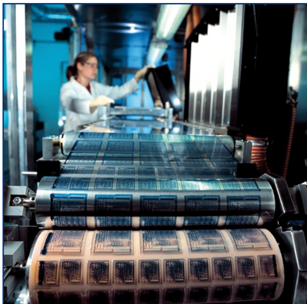
Figure 4. Polymer circuits can be manufactured at speeds of up to 20 m per minute using conventional printing machines. (Photograph: PolyIC)
